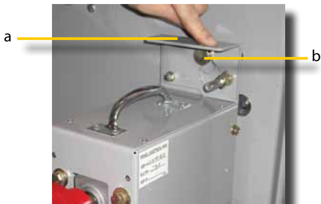
Figure 18 Push Down the Support Latch
