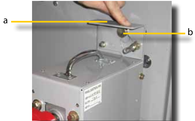
Figure 10 Push Down the Support Latch
